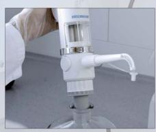
Ground adapter for direct reagent extraction from a ground bottle.
