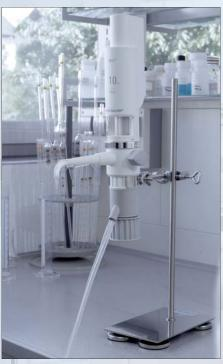
Stand clip for fixing the basic unit.
